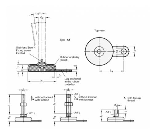
$\begin{array}{ll} A/F1 = 17 \\ d1 &= 60 \\ d2 &= M8 \\ h1 &= 19 \\ h3 &= 27 \\ l1 &= 50 \\ l8 &= 25 \\ l9 &= 50 \end{array}$
